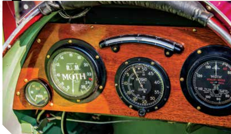
No, the skidball is not upside down: it's a bubble level and, like everything else in the airplane, is original.
