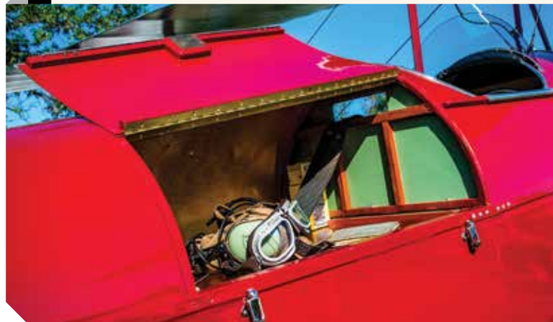
The baggage compartment reveals the totally wooden nature of the fuselage.
